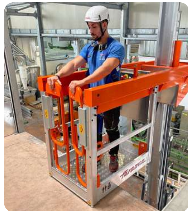
Elevah speciale per sbarco in quota. Special Elevah designed to exit the platform at height.
