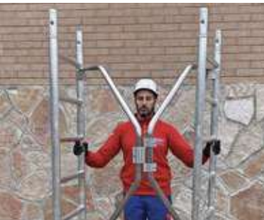
Base con kit richiudibile standard. Base with folding kit.
